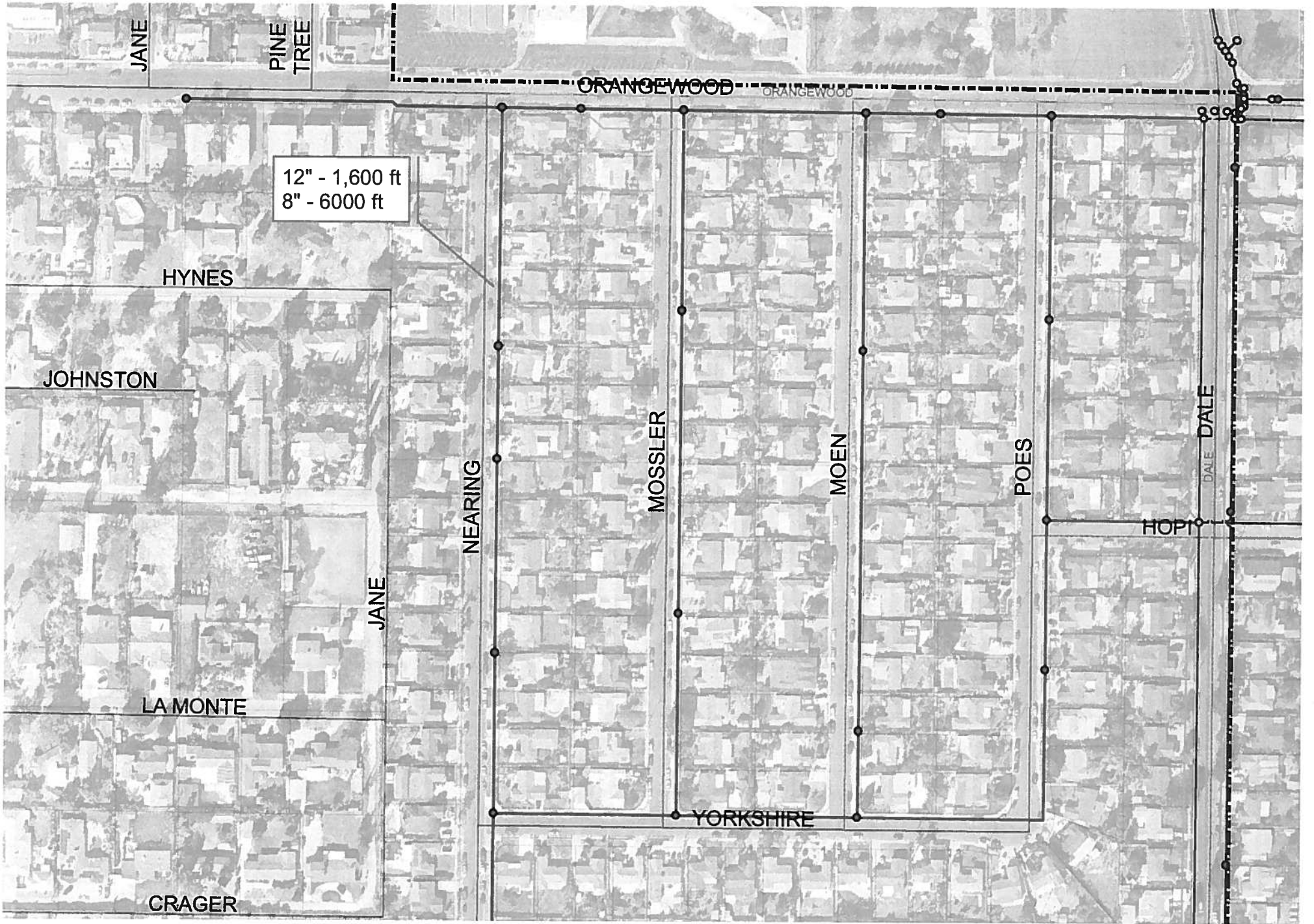
Small Diameter Upsize: Orangewood Dr and Dale St Water Replacment Project
